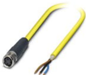
Sensor/actuator cable, 3-position, PVC, yellow, shielded, free cable end, on Socket straight M8, cable length: 5 m
