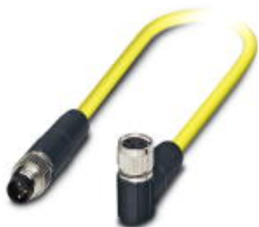
Sensor/actuator cable, 3-position, PVC, yellow, shielded, Plug straight M8, on Socket angled M8, cable length: 0.5 m
