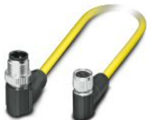
Sensor/actuator cable, 3-position, PVC, yellow, shielded, Plug angled M12 SPEEDCON, coding: A, on Socket angled M8, cable length: 1.5 m
