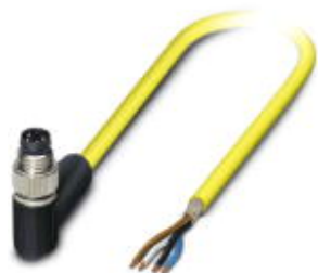
Sensor/actuator cable, 4-position, PVC, yellow, shielded, Plug angled M8, on free cable end, cable length: 2 m
