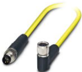
Sensor/actuator cable, 4-position, PVC, yellow, shielded, Plug straight M8, on Socket angled M8, cable length: 0.5 m
