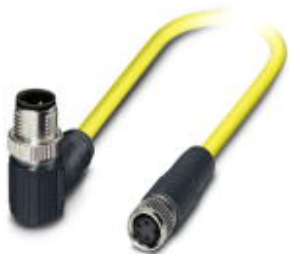
Sensor/actuator cable, 4-position, PVC, yellow, shielded, Plug angled M12 SPEEDCON, coding: A, on Socket straight M8, cable length: 1.5 m
