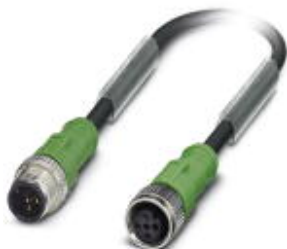
Sensor/actuator cable, 3-position, PUR halogen-free, black-gray RAL 7021, Plug straight M12, coding: A, on Socket straight M12, coding: A, cable length: 10 m, For valve connector
