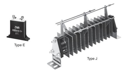
"ZNR" Transient/Surge Absorber for thyristors is especially designed to protect SCR power controllers and SCR power sources from high energy transient over voltages.
