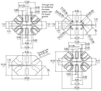
SMA connector to be soldered
