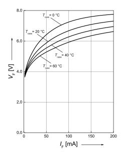
**Opt. Power / Forward Voltage** <sup>6), 7)</sup> B2:  $V_F = f(I_F)$ ;  $T_{case} = 25^{\circ}C$
