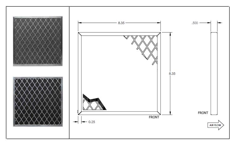
Orion Fans Hydrophobic Mesh air filters are water-repellent and offer a low pressure drop, cost-effective solution. The combination of hydrophobic mesh on the downstream side and high density foam on the upstream side offers a durable, cleanable, and moisture-resistant product. Designed for outdoor cabinets, process equipment applications requiring mist elimination, or other harsh environment installations.
