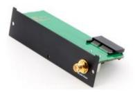
The Monnit® expansion card inserts into the back expansion slot of the CloudGate and allows the CloudGate to function as a gateway for wireless Monnit® devices like sensors and relays over the 433MHz, the 868MHz or the 900MHz band. Monnit® Wifi sensors are not supported.
