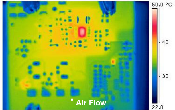
Figure 35. Thermal Image of the Bottom of the Board at Low Line and Full Load Condition
