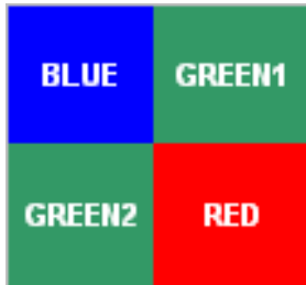
Figure 3. Color Filter Arrangement on the Pixels
