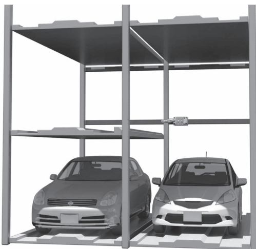
Detection of Car Pallet Positions in Parking Towers
