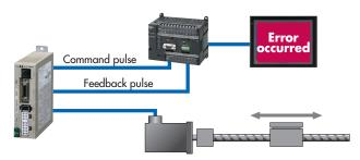
Simplified Sychronization: It is also possible to input encoder output signals directly into the servo drive.
