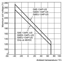
Note: The maximum coil voltage refers to the maximum value in a varying range of operating power voltage, not a continuous
