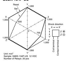
Test Conditions: Shock is applied in ±X, ±Y, and ±Z directions three times each with and without energizing the Relays to check the number of contact malfunction.
