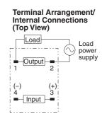
Terminal Arrangement/ Internal Connections (Top View)
