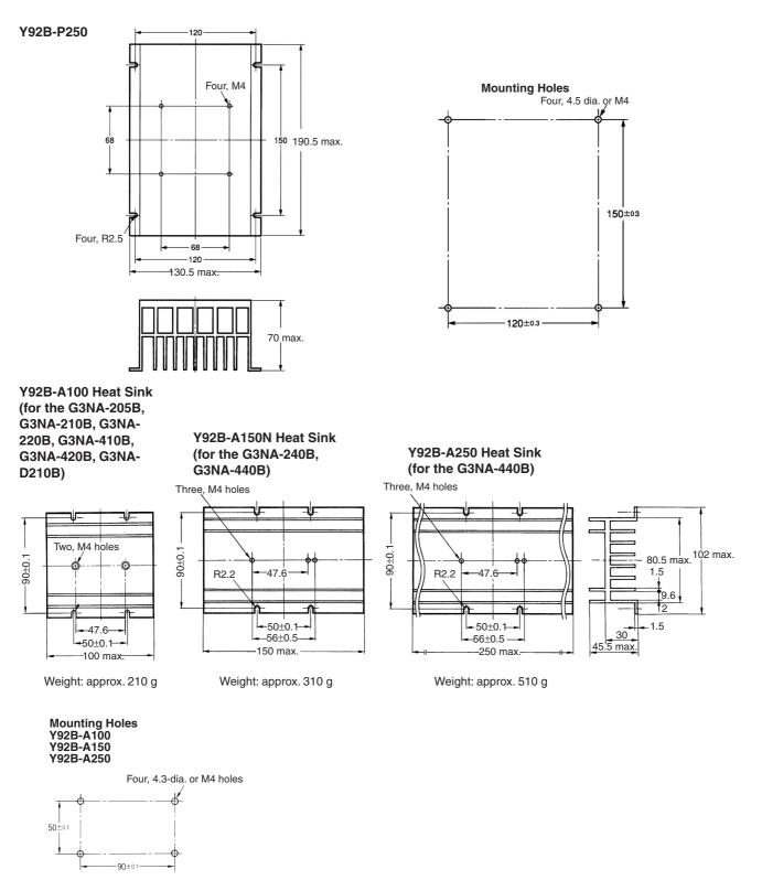
For surface mounting, a 30% derating of the load current is required (from the Load Current vs. Ambient Temperature graphs). The orientation indicated by the external dimensions is not the correct mounting orientation. When opening mounting holes, refer to the mounting hole dimensions.
