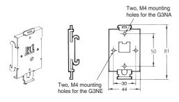
To mount the Relay to DIN Track, first mount it to the One-touch Mounting Plate and then attach it to the DIN Track as shown in the diagram. To remove the Relay from the DIN Track, pull down on the tab with a screwdriver in the direction of the arrow.
