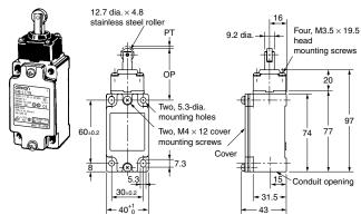
Note:Omitted dimensions are the same as those for the Roller Lever Type Models. D4B-1□□□N and D4B-5□□□N have a PG13.5 conduit opening. D4B-2 \Bullet \Bullet N and D4B-6 \Bullet \Bullet N have a G1/2 conduit opening. D4B-3□□N and D4B-7□□N have a 1/2-14NPT conduit opening.
