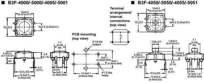
\* Fit the projection of the switch into this hole to secure the switch.
