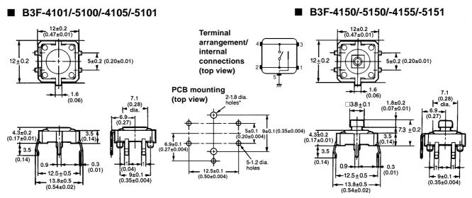
\* Fit the projection of the switch into this hole to secure the switch.
