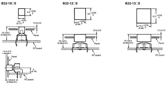
Note: 1. Unless otherwise specified, a tolerance of  $\pm$  0.2 mm applies to all dimensions.
