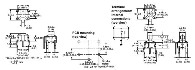
Terminal numbers are not indicated on this switch. With the switch turned over so that the logo mark "OMRON" is visible on the upper part of the rear Note: side of the switch base, the terminal on the right of the logo mark is numbered "1" and that on the bottom right is "3." Accordingly, two terminals on the left side are numbered "2" and "4" respectively.
