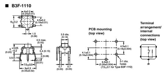
Note: Terminal numbers are not indicated on this switch. With the switch turned over so that the logo mark "OMRON" is visible on the upper part of the rear side of the switch base, the terminal on the right of the logo mark is numbered "1" and that on the bottom right is "3." Accordingly, two terminals on the left side are numbered "2" and "4" respectively.
