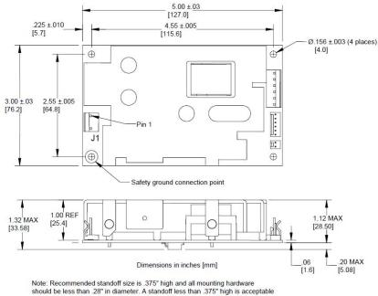
Note: Recommended standoff size is .3/5° high and all mounting hardware should be less than .28" in diameter. A standoff less than .375" high is acceptable when a thin insulator, 0.4mm thick (polyester, fish paper or equivalent UL rated 94V-2 minimum) is placed between the XL160 and the mounting chassis (refer to applicable UL standard for clearance requirements).
