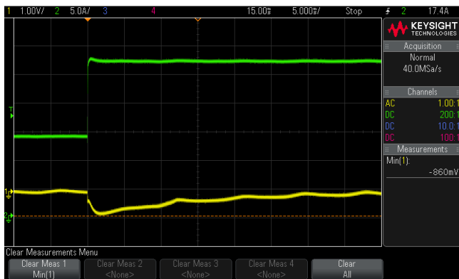
Inrush Current; 264Vac Input, Cold Start, 10.5Apk
