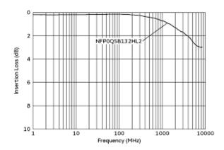
Common Mode Insertion Loss Characteristic (Typical Value)
