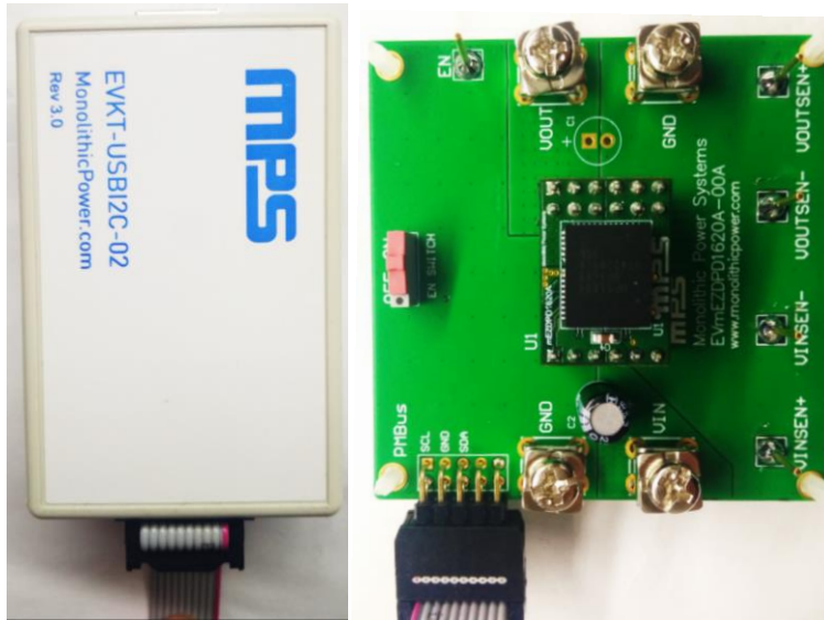
Figure 5: EVB to MPS I 2 C Communication Interface Wire Connection
