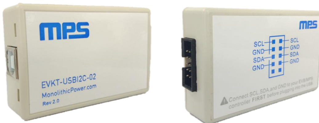
Figure 3: EVKT-USBI2C-02 Communication Interface Device
