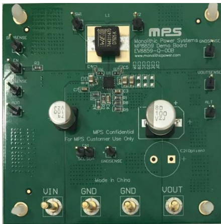
Figure 2: EV8859-Q-00B Evaluation Board
