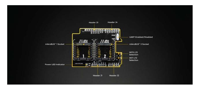
LCPXpresso Click Shield designed to support multiple NXP platforms which use Arduino connector and equip them with two mikroBUS sockets. This shield is specially designed with high attention to specific of the LPCXpresso pinout, which is slightly distinguishable from the classic Arduino pinout. For this we have provided additional switches which allows you to select digital I/O on the interrupt pins (INT0/INT1).
