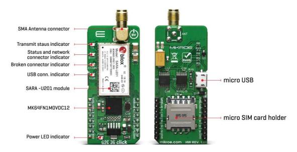
G2C 3G click performs several tasks on its side, which are required to connect to the Click Cloud platform. To establish the connection, an access to a local UMTS/HSPA network with sim card option. For a reliable 3G (UMTS/HSPA) network connection, the Click board<sup>™</sup> utilizes the u-Blox SARA U-201 module can be used worldwide.
