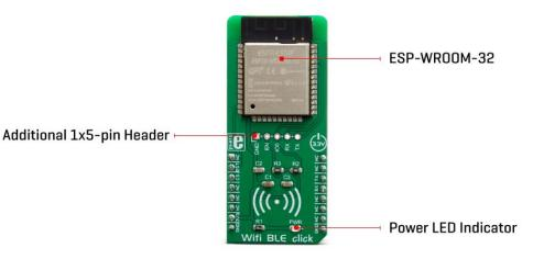
The ESP32-WROOM-32 supports 802.11 b/g/n WiFi standards at 2.4GHz, allowing up to 150Mbps for the 802.11n. Security options including WEP, WPA/WPA2 PSK/Enterprise, as well as hardware accelerated encryption including the AES/SHA2/Elliptical Curve Cryptography/RSA-4096, are also present on the ESP32-WROOM-32 module. It supports Sniffer, Station, SoftAP, and Wi-Fi direct modes. The ESP32-WROOM-32 module also complies with the Bluetooth v4.2 BR/EDR, and BLE specifications.
