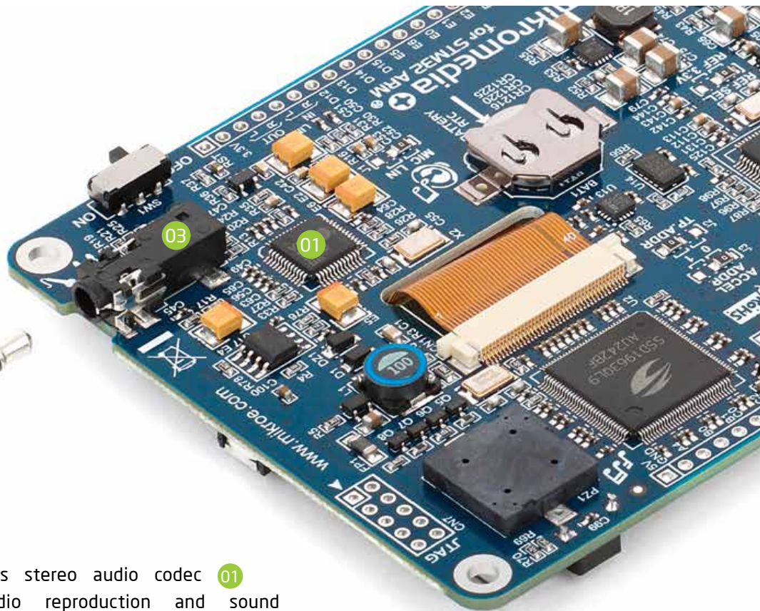
Figure 8-1: On-board VS1053 MP3 codec
