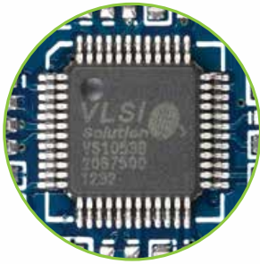
Figure 8-1: On-board VS1053 MP3 codec
