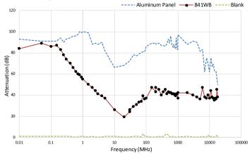
Test performed with a two-coat thickness.
