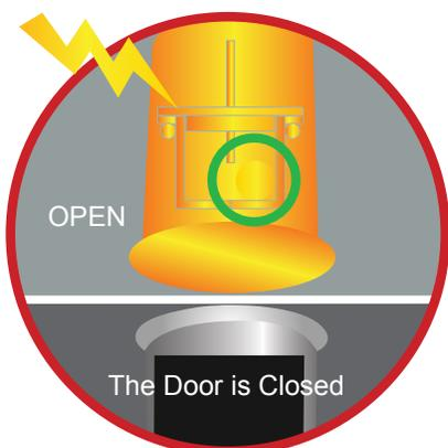
MAGNASPHERE Security Sensors are highly resistant to contact welding from power surges and lightning strikes.
