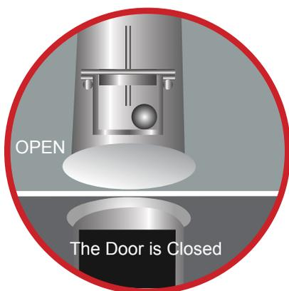
MAGNASPHERE security sensors' magnet ball contact is open in the secure position (Open Loop) when the door is closed and the door magnet is near the switch.
