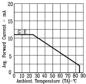
Fig5. MAX. AVERAGE FORWARD CURRENT VS. AMBIENT TEMPERATURE.
