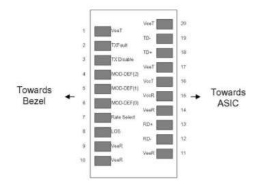
Pin-out of connector Block on Host board
