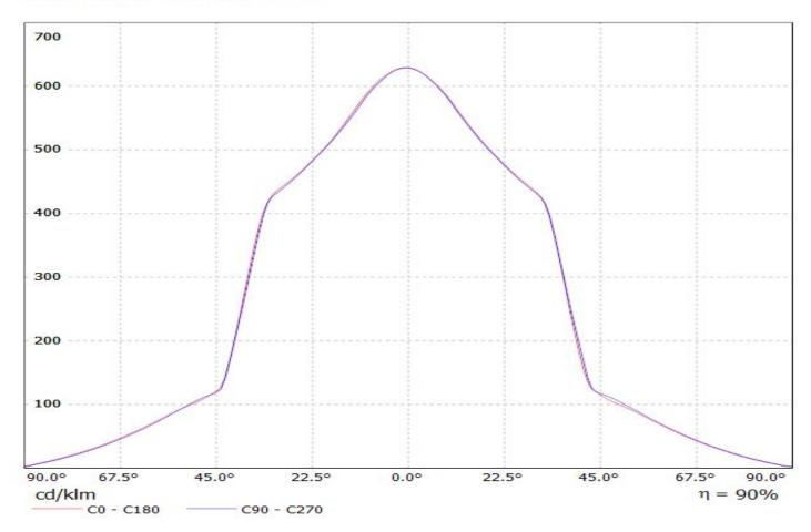
Luminaire: Ledil Oy CN12647\_LENINA-S-DL (Megazenigata 867lm @ 250mA) Efficiency=82% Lamps: 1 x Megazenigata 867lm @ 250mA
