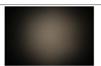
LED LH181A **FWHM** 28.0° Efficiency 80 % Peak intensity 2.6 cd/lm LEDs/each optic 1
