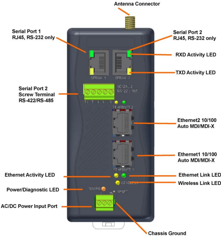
Figure 4-6. XPress DR+W Front Panel Layout
