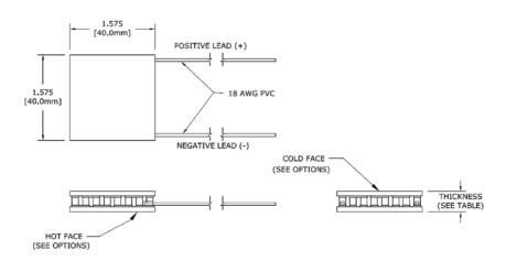
Ceramic Material: Alumina (AI<sub>2</sub>O<sub>3</sub>)
