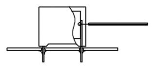
Temperature monitored inside the capacitor.
