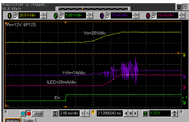
FIGURE 14. IN-RUSH and LED CURRENT AT V_{IN} = 12V FOR 6P12S AT 20mA/CHANNEL
