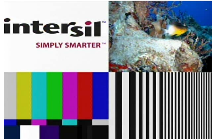
FIGURE 10. TEST PATTERN IMAGE AFTER 3000 FEET OF CAT 5 WITH ISL59603 (OR BETTER)
