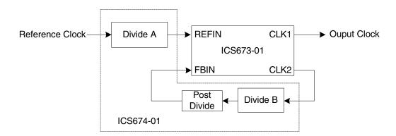
If the reference is in the kHz range, for example 8 kHz, the following configuration may be more typical:
