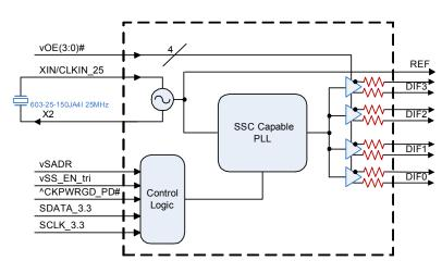
Note: Resistors default to internal on 41/51 devices. P1 devices have programmable default impedances on an output-by-output basis.
