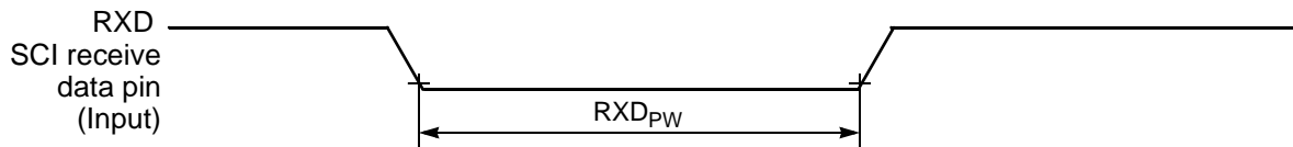
Figure 10-16 RXD Pulse Width
