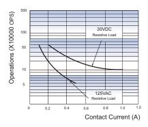
**Test conditions:** Resistive load, at 85°C, 1s on 9s off.
