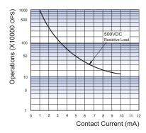
**Test conditions:** Resistive load, at 105°C.
