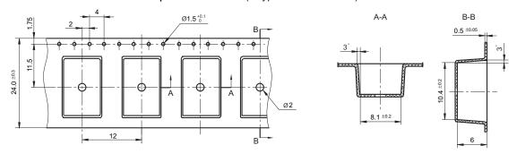
TAPE PACKING Unit: mm
