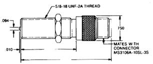
Sensors with 5/8-18 UNF-2A mounting thread, AWG 22 PVC shielded cable (1,65 m [65 in] long), 10 kHz typical frequency response
