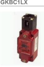
GK Series, Key Operated Safety Interlock Switch, 1NC/1NO Direct Opening, Snap Action, 20 mm, Zinc Die cast Housing, Silver Contacts
