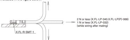
When the cable is routed in such a direction that lifts the cable, it is recommended that cushioning should be placed on the plug to prevent the connector from unmating (see the example below).
