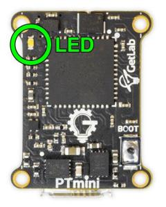
**LED:** When plugged in to micro-usb power and a Lepton is inserted in the socket LED will flash slowly. When video is being transmitted to the viewing program, LED will flash more rapidly
