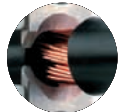
Round stripping blades on Pro 16 cut insulation cleanly
