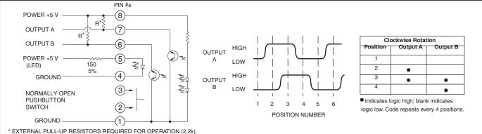
\*\* Circuit shown with on-board lighting system. Versions without on-board lighting system do not have LED power connections. Refer to standard 62A series for circuitry.
